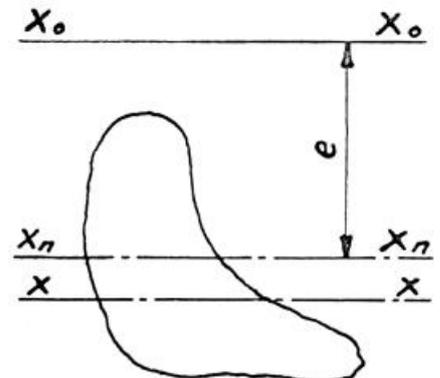
Large diagrams exceeding the range of the tracing point must be cut into smaller portions. If it is found impossible to follow the single portions with the tracing point after setting the rail of the Integrator to the axis of moments, an auxiliary axis parallel to the original axis of moments must be drawn for each portion.
