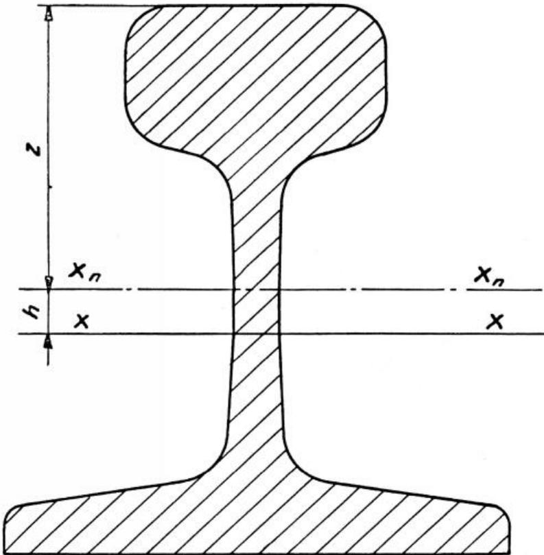
Set off the neutral axis  $x_n - x_n$ , adjust the rail to the line  $x_n - x_n$  as the new axis of moments, and again circumscribe the profile by means of No. 2 tracing point, taking readings on all the rollers. Thus:
