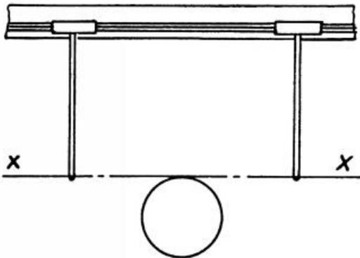
This shows that the A and I rollers perform the same travel whether the diagram lies inside or outside the axis, but that the M roller moves in the opposite direction in the latter case. The travel must then be taken into account as a negative quantity.
