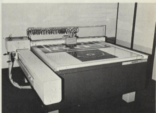
Coradomat—Producing photomasks on peelcoat on a time-sharing basis at Thomas L. Faul Assoc. Inc., Skaneateles, N.Y.
