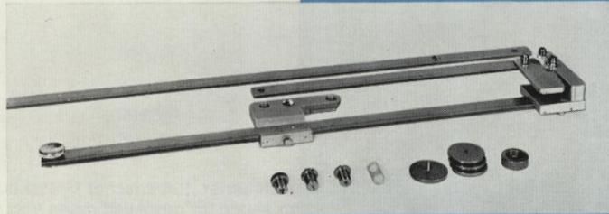
Accessories are available for drafting with pencil, ball pen, inking pen, Rapidograph pens, sapphire scribes and cut and peel foil knives. Reading microscope and pricker point and reading microscope for readout of coordinates. The Coradograph beam compass used for circular and radial lines or cuts up to 23  $\frac{5}{8}$ " radius (or 600 mm R).
