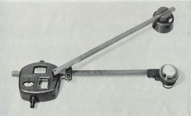
range is within 28 in. dia circle. Type Core-Junior is a high precision planimeter with fixed arm lengths and normal vernier reading dials.
